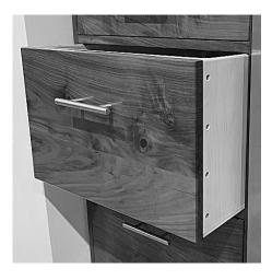
What I built are stable drawers with pre-finished surfaces, a snug fitting and slippery bottom, tidy screw positions along the side corners, and counter-sunk screws up from the bottom into the verticals. There was no lost space or extra cost for hardware. I did round over the top
